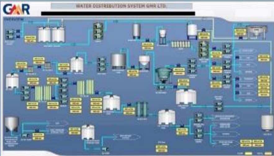
SCADA for water accounting -3.17 Lac m3 savings
